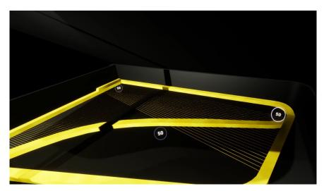
Each sound source has a ring that provides a real-time visual representation of the source's relative amplitude by changing its size. The opacity of the ring is reduced when a sound source is muted. The number in the middle represents the source's absolute volume with a range of 0 to 100. The number and ring constantly rotate to face the user in order to enhance their visibility inside the 3D virtual environment.
